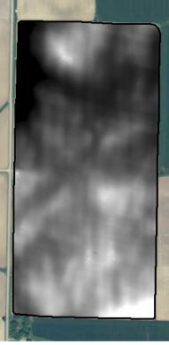
LiDAR elevation to extent of field
