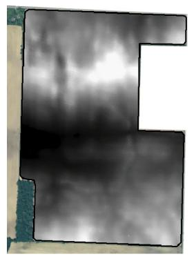
LiDAR elevation to extent of field
