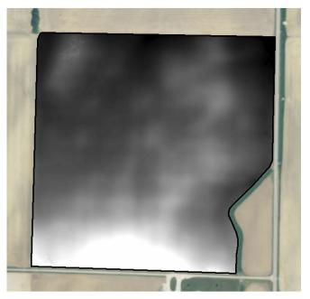
LiDAR elevation to extent of field
